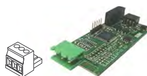
Figure 24 - Detail of the 'S4' RS-485 communications module
